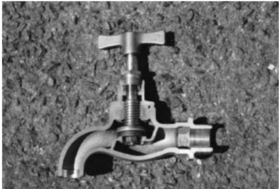
Figure 5.3.2: A cross section through a tap
